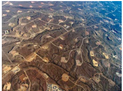
Figure 2 Aerial view (B. Gordon, EcoFlight) of hydraulic fracturing pads. Looking north across part of the Jonah tight gas field (of Late Cretaceous age) in Wyoming.
