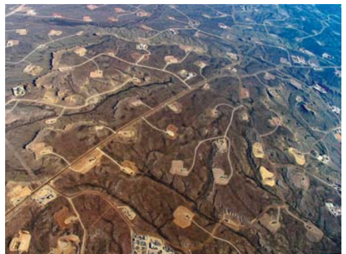
Figure 2 Aerial view (B. Gordon, EcoFlight) of hydraulic fracking pads. Looking north across part of the Jonah tight gas field (of Late Cretaceous age) in Wyoming.
