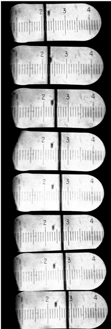
This figure shows photographs looking into the eyepiece of meter G-275 as it is balanced. The reading line of this meter is 2.70. Here, the cursor reads 2.1, so we need to turn the dial to the right ...
