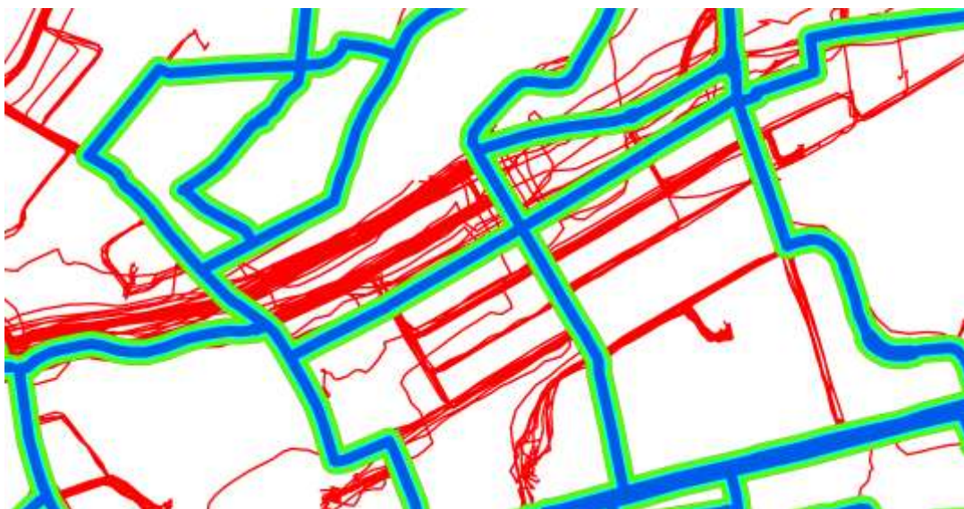
Figure 3: Corridor space definitions using a map: 10m Blue buffer equals cycle trips on network, 10 green buffer equals close to network trips and red is for cycle trips off the
