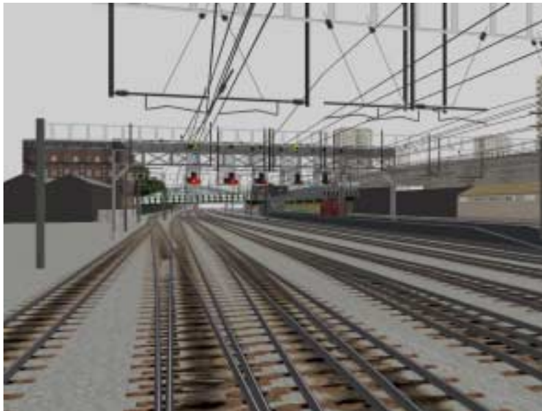
SolvSIGHTING accurately models all signals, furniture, rail traffic, lighting and visibility conditions. The positioning of signals, structures and furniture can now be ‘optioneered’ during the design process, to minimise and sighting problems before on-site signal sighting reviews are undertaken.
