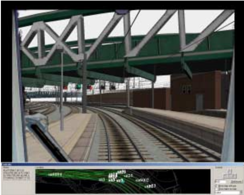
The driver's view in solvRL. All signaling is event-driven, with a realistic cab's-eye view of the approaching track and surrounding structures, seamlessly animated as the train moves forward. Behind solvRL sits the entire mapping base for the UK rail network; the lower display shows the 'virtual train's' real life position.
