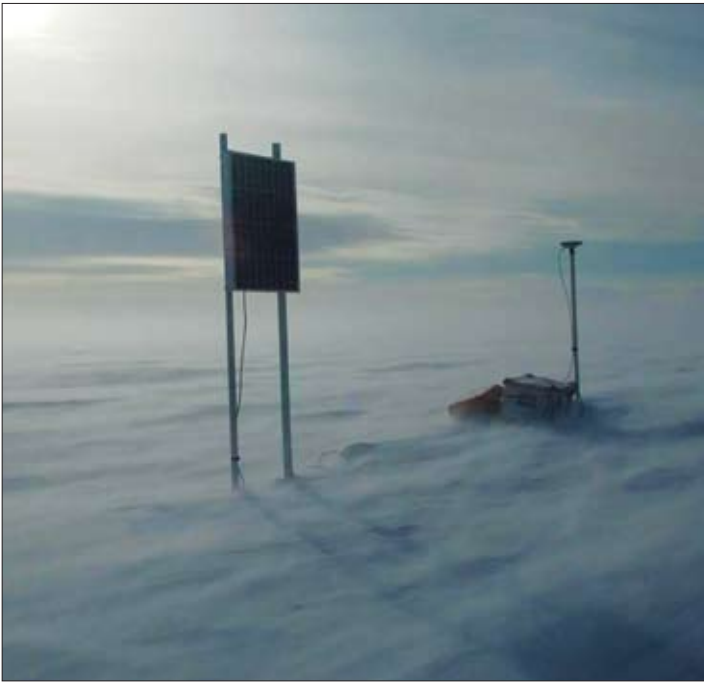
4: Glacier seismic and GPS station on the West Antarctic Ice Sheet. (A Smith)
