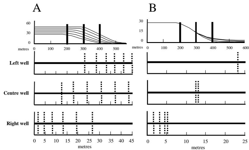
*Fig. 3. Sections of different parasequences sampled at a well are approximately equivalent to sections of the same (e.g., lowermost) parasequence taken at successively horizontally offset locations. Intersections refer to the parasequence boundaries; Available cross sections are horizontally offset points where parasequence thicknesses occur that are equivalent to those found in the well. The double arrows indicate to which well section each available cross section is similar.*
