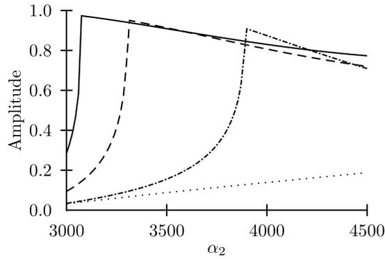
**Figure 7.** Reflected P wave amplitude data as a function of parameter  $\alpha_2$  for four different offsets:  $x = 500$  m (dotted line),  $x = 1000$  m (dot-dash line),  $x = 1500$  m (dashed line), and  $x = 2000$  m (solid line). The velocity of the top layer is  $2750 \text{ m s}^{-1}$ , and the depth to the reflecting boundary is  $500$  m.
