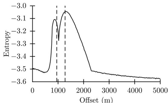
**Figure 9.** Entropy values as a function of offset for a two-receiver experimental design using the iteratively constructive method with the first receiver fixed at 1050 m. The entropy at each offset is calculated using 500,000 samples and a data space discretization of 0.01. Entropies are calculated at offsets ranging from 0 m to 5000 m at 25-m intervals. The dashed lines represent the optimal offsets found by searching the complete design space (Figure 10).
