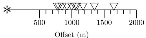
**Figure 14.** Experimental design using 10 receivers placed using the iteratively constructive method and 500,000 parameter-space samples. The source is denoted by asterisk and each receiver by an inverted triangle.
