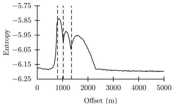
**Figure 11.** Entropy values as a function of offset for a three-receiver experimental design using the iteratively constructive method with the first two receivers fixed at offsets of 1050 and 1350 m. The dashed lines represent the globally optimal three-receiver design (Figure 12).
