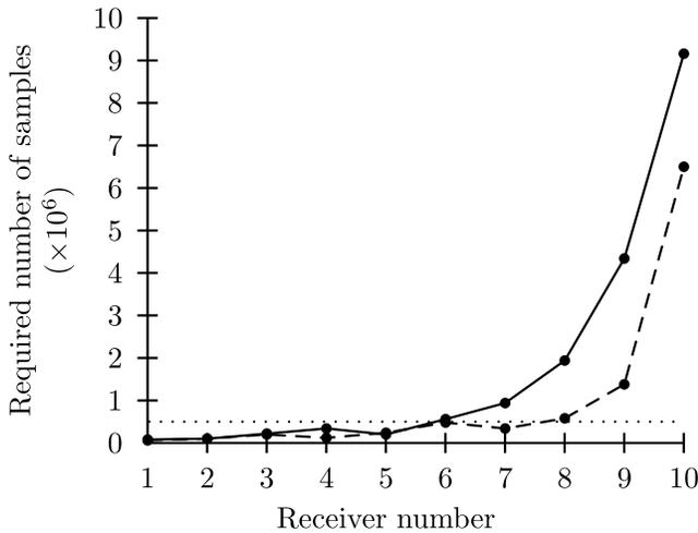
**Figure 17.** The number of samples required to accurately locate the optimal receiver using the iteratively constructive method to 95% (solid line) and 66% (dashed line) confidence. The dotted line shows the number of samples used in our previous example (Figure 14); we had oversampled the first five experiments but undersampled the final five.
