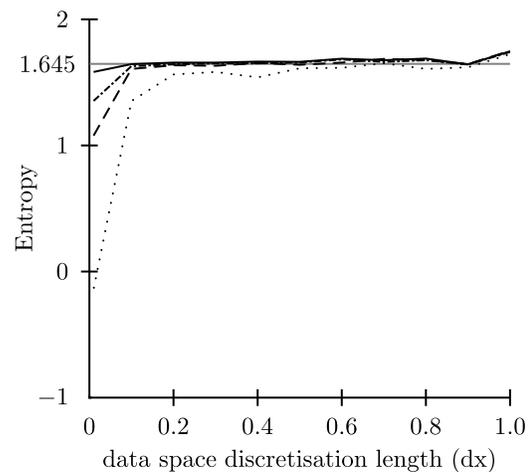
**Figure 3.** Entropy values for the single-period sawtooth function as a function of data space discretization length ( $dx$ ) for four experiments with different numbers of parameter space samples (dotted, 100; dashed, 500; dot-dashed, 1000; solid, 5000). The gray line represents the analytical value of 1.645.
