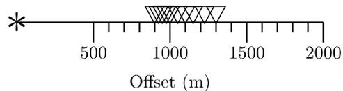
**Figure 19.** Experimental design using 10 receivers placed using the iteratively constructive method with the variable sample size test and a reduced prior parameter range. The source is denoted by asterisk, and each receiver is denoted by an inverse triangle.
