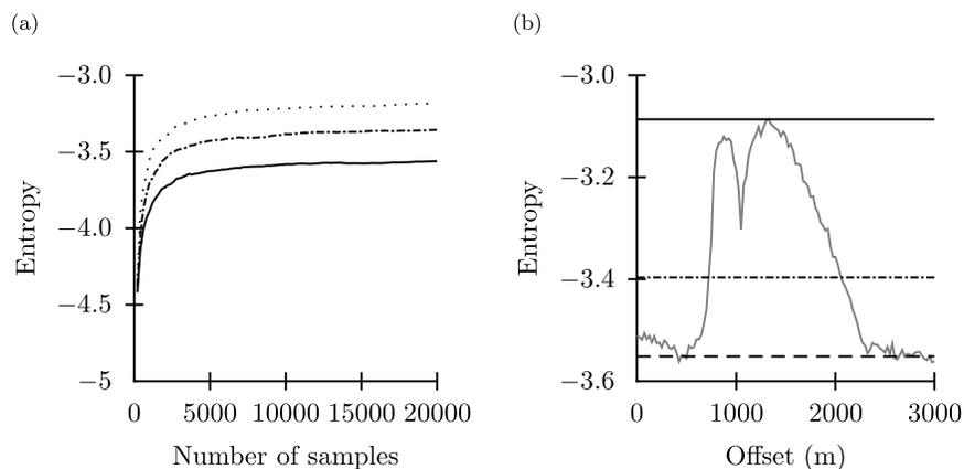
**Figure 15.** (a) The entropy estimates for offsets of 1000 m (dotted), 2000 m (dot-dash), and 3000 m (solid), as increasing number of samples are drawn from the parameter space. (b) The resulting entropy profile (gray line) produced from 20,000 samples. The solid line indicates the maximum entropy value, the dot-dashed line indicates two standard deviations, and the dashed line indicated three standard deviations from the maximum.
