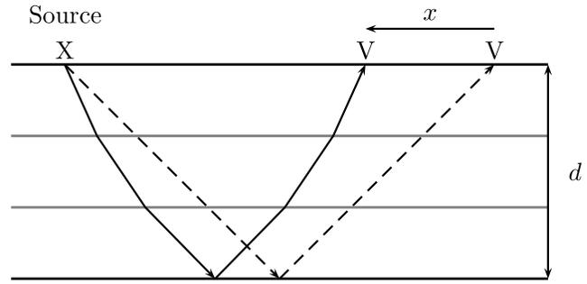
**Figure 18.** Raypath differences caused by having a different subsurface model. The dashed line represents a model with no refraction before the targeted interface, whereas the solid line refracts at two interfaces (gray lines), both before and after reflection. Both raypaths have the same angle of incidence and reflection at the lower-most interface.
