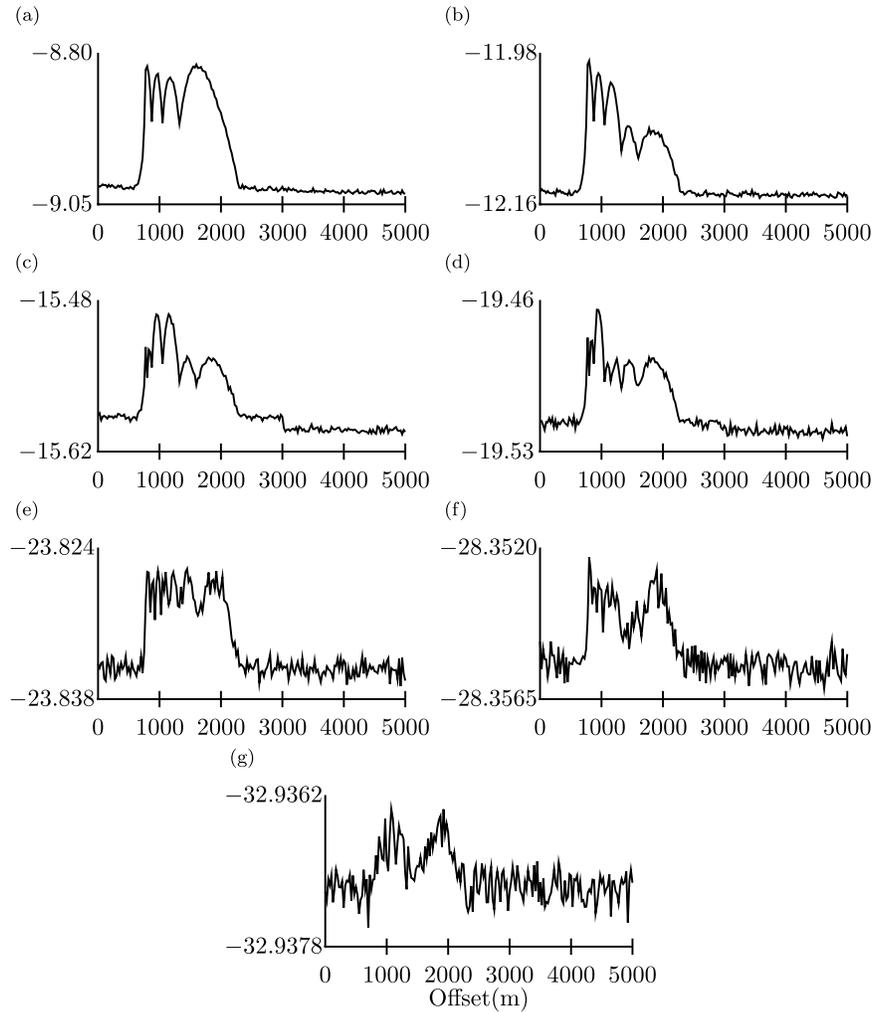
**Figure 13.** Entropy plots for successive receiver locations using our iteratively constructive method. (a) The entropy curve used to place the fourth receiver, and (g) the curve used to place the tenth receiver. For each plot, 500,000 parameter samples are used and the discretization length in each data-space dimension is 0.01.
