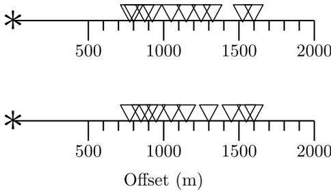
**Figure 16.** Experimental design using 10 receivers placed using the iteratively constructive method with the variable sample size test. Top design represents optimal 10-receiver design to 95% confidence and lower design to 66% confidence.
