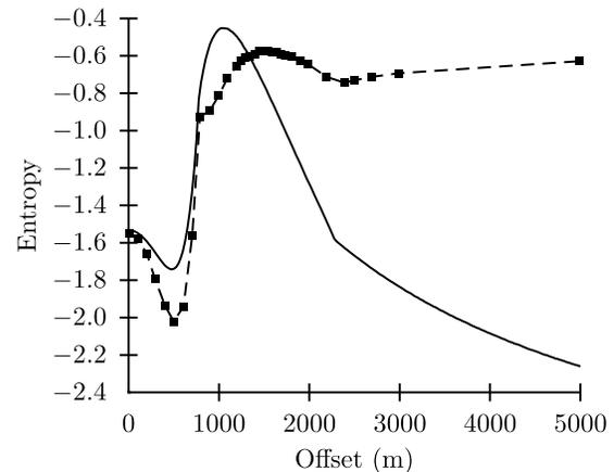
**Figure 8.** Entropy values as a function of offset for a single receiver. The most densely sampled results of *van den Berg et al.* [2003] are represented by the dashed line (data space discretization length of  $0.001$  using  $300,000$  samples). The solid line represents our results using a data discretization length of  $0.01$  using  $500,000$  samples.
