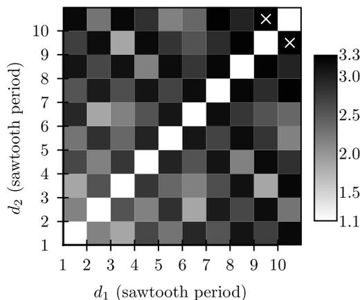
**Figure 5.** Two-data entropy values of entropy of  $\sigma(\mathbf{d})$  for the complete design space for pairs of sawtooth functions with integer periods ranging from 1 to 10 over the parameter range of 0–10. For each experiment, the data space discretization length is 0.1 and 500,000 samples are drawn at random from a Uniform prior distribution over the parameter range. The white crosses indicate the optimal two-data experimental design.
