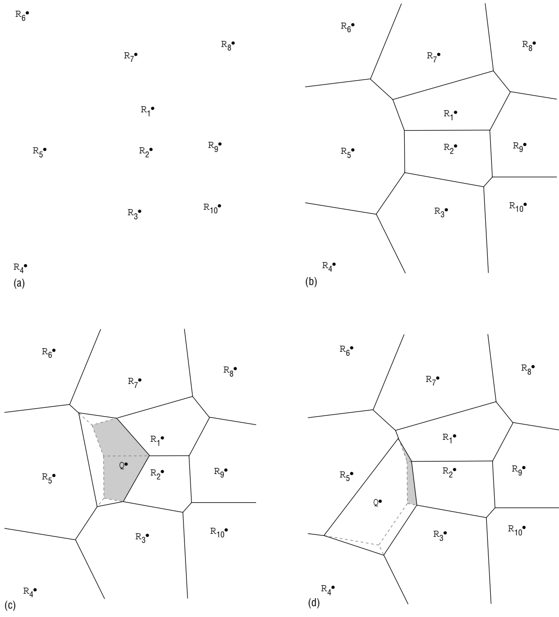
Fig 19. (a) Set of reference points; (b) Ordinary Voronoi diagram of reference points; (c) and (d) Ordinary Voronoi diagram of reference points and query point Q for two different locations of Q .
