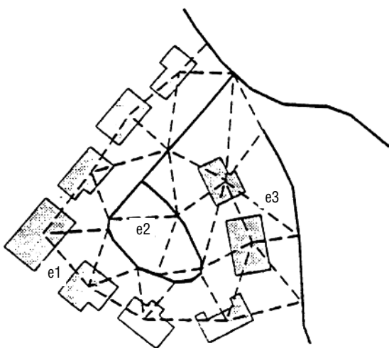
Fig 9. Local Delaunay triangulation between buildings and adjacent roads (after Ruas 1995a).
