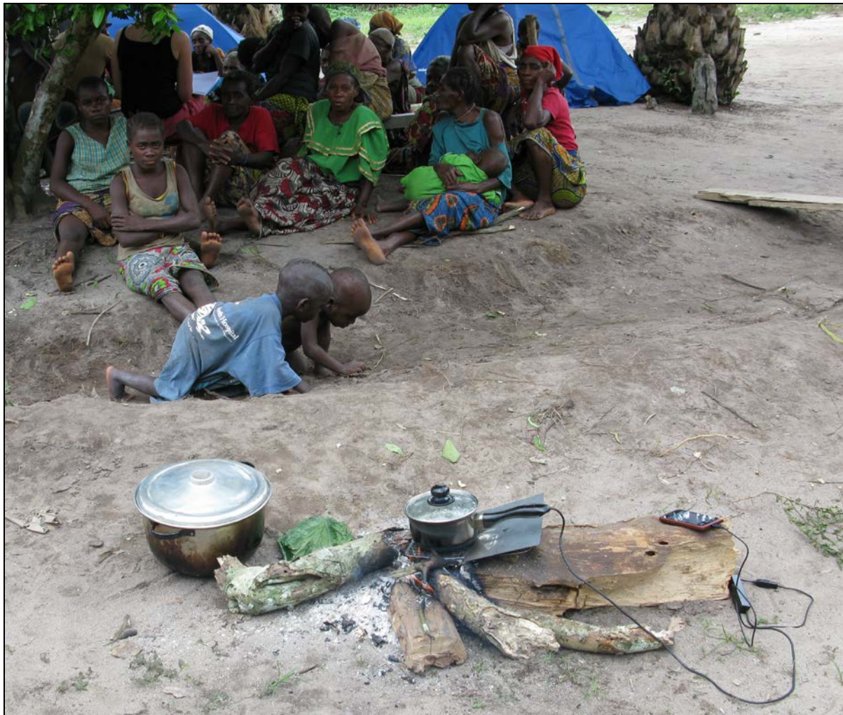
Figure 2. Charging a phone with pan charger
