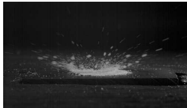
Figure 5. Image of splash from 4 mm drop on fine sand approximately 0.02 s after initial impact, showing ejected grains and grain clumps.
