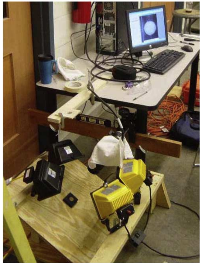
Figure 1. Experimental setup showing inclined board with sand target (black), high-wattage lighting, high-speed camera (covered by towel), and computer image of target. Sand target has diameter of 2.5 cm and depth of \sim 2 cm; experiments with sticky paper involve placing the paper ( \sim 2 cm diameter holes) over the sand target such that the sand surface is flush with the paper surface.
