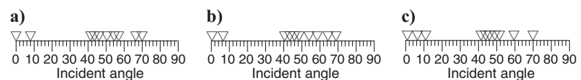
Figure 9. Processing design using 10 receivers placed using the Guest and Curtis (2009) method allowing only incident angles as high as 70^\circ . Plot (a) represents the final design for a brine-filled reservoir, (b) an oil-filled reservoir, and (c) a gas-filled reservoir.
