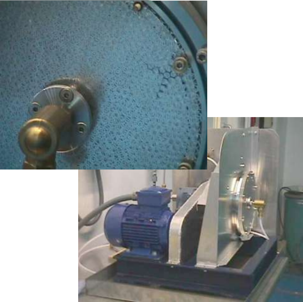
Spinning Disc Reactor used to study bubble and mass transfer performance
